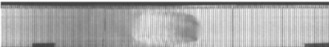
Scanning moiré of a dented can
